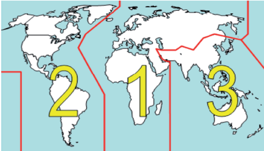
Figure 5.23. For the purpose of Radio Regulations, the world has been divided into three geographical regions numbered 1, 2, and 3.
